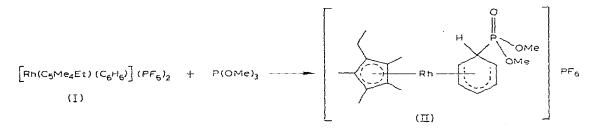
Microanalysis of the yellow crystalline product is consistent with the proposed formulation (Found: C, 39.1; H, 4.8.  $C_{19}$  H<sub>29</sub> F<sub>6</sub> O<sub>3</sub> P<sub>2</sub> Rh calcd.: C, 39.1; H, 5.0%). Integration of the <sup>1</sup>H NMR spectrum confirmed that only two methoxy groups were present and both the <sup>13</sup>C and <sup>1</sup>H NMR spectra were characteristic of a cyclohexadienyl compound (Table 1). Evidence that
